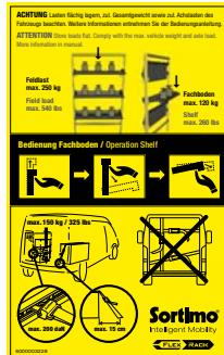
These safety markings are located on the divider of your vehicle. The safety marking indicates the maximum load capacity of a shelf, as well as showing how to use the FlexRack.
